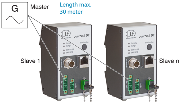
Fig. 29 Synchronization of multiple controllers, star-shaped
