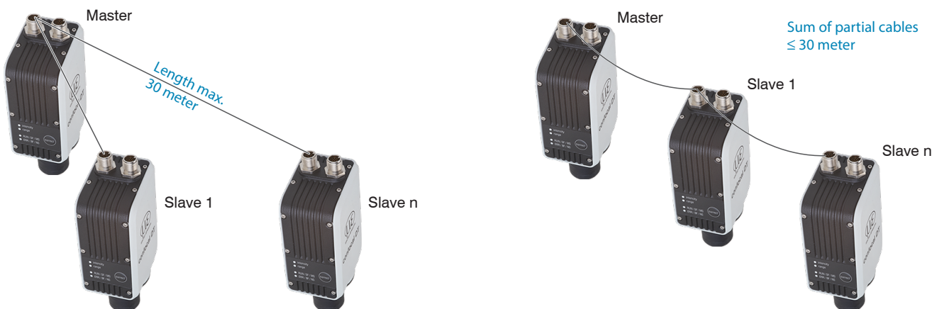
Fig. 14 Synchronization of multiple sensors, star-shaped on the left, daisy-chained on the right
