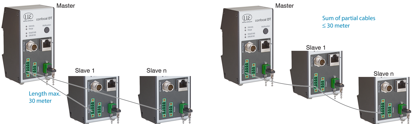
Fig. 27 Synchronization of multiple controllers, star-shaped on the left, daisy-chained on the right
