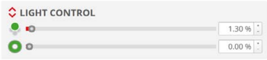
Light Control in Inspection Settings, also showing the controls for the optionally available ring light
