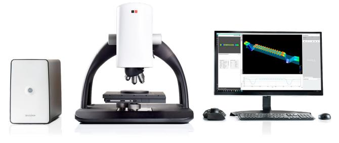
The sample is placed under the objective lens held by a motorized nosepiece and on the top of a manual or a motorized XY stage and a manual tip-tilt.
