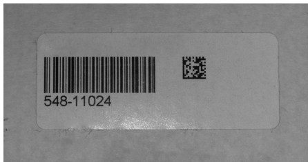
Fig. 238: Comparison of DataMatrix code and barcode
