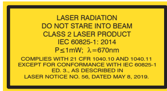
Fig. 1 Laser labels on the sensor cable
