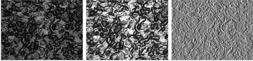
Examples of filters: (a) Harsh, (b) Sobel and (c) Prewitt
