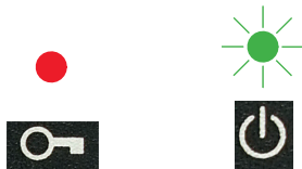
Fig. 16 Green LED flashing, red LED illuminated continuously
