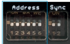
Fig. 59 DIP switch on the MSC7602 for multi-channel operation
