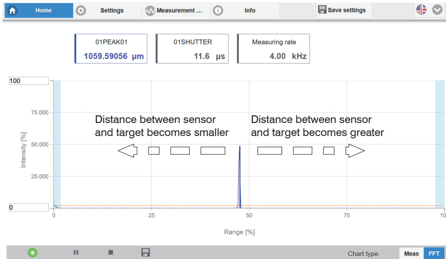
Fig. 25 Using the FFT signal for sensor positioning
