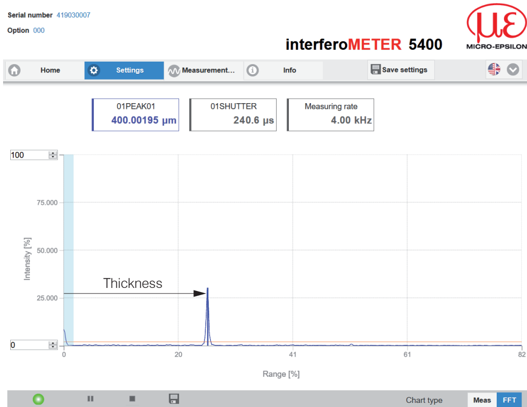
Fig. 59 FFT signal web page (thickness measurement)
