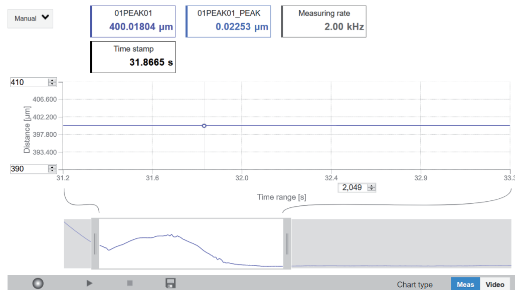
Fig. 60 Offline analysis of measured thickness results based on a one-sided thickness measurement
