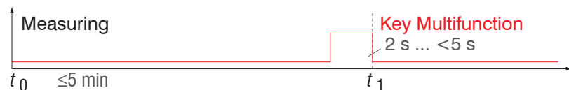
Fig. 49 Flow chart for resetting zeroing/mastering
