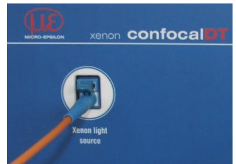
Fig. 16 Connecting the optical fiber to IFX2471
