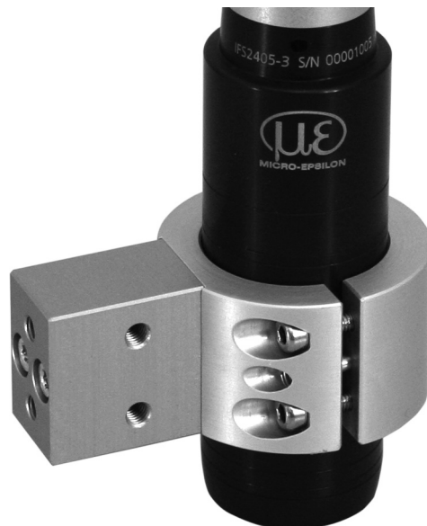
Fig. 22 Outer clamps with installation bracket MA240x for IFS2405, IFS2406 and IFS2407 sensor, consisting of mounting block and mounting ring
